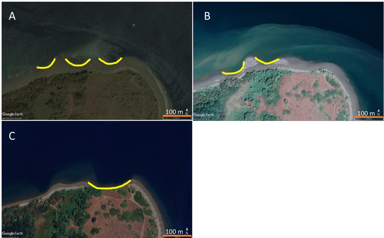
Figure 4. Remaining evidence of three events mapped on Google Earth imagery. Yellow lines mark the evidence of scarp crowns that are visible in the images. A) The February 9 th , 2008 event, in which three scarp crowns are visible: the one on the right is located at the same site as the February 2024 event, although it is smaller, while the other two on the left are in similar positions to the scarps observed in the 2017 event. B) Marks the evidence of the January 27 th , 2017 event, showing two crowns, one to the left and the other toward the center, although it is unclear whether one occurred at the same location as the February 2024 event. C) The February 8 th , 2024 event, captured in an image taken on March 7 th , 2024. Source: Google Earth (2008, 2017, 2024).
