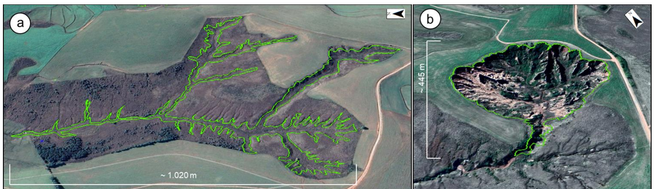
Figure 15. Examples of gullies integrated with the drainage network. Adapted from Google Earth Pro (2024).
