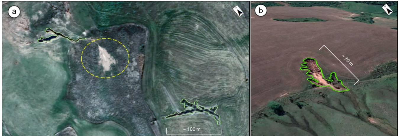
Figure 14. Examples of gullies disconnected from the drainage network, with a circle indicating a fan of sediment transported by runoff action. Adapted from Google Earth Pro (2024).
