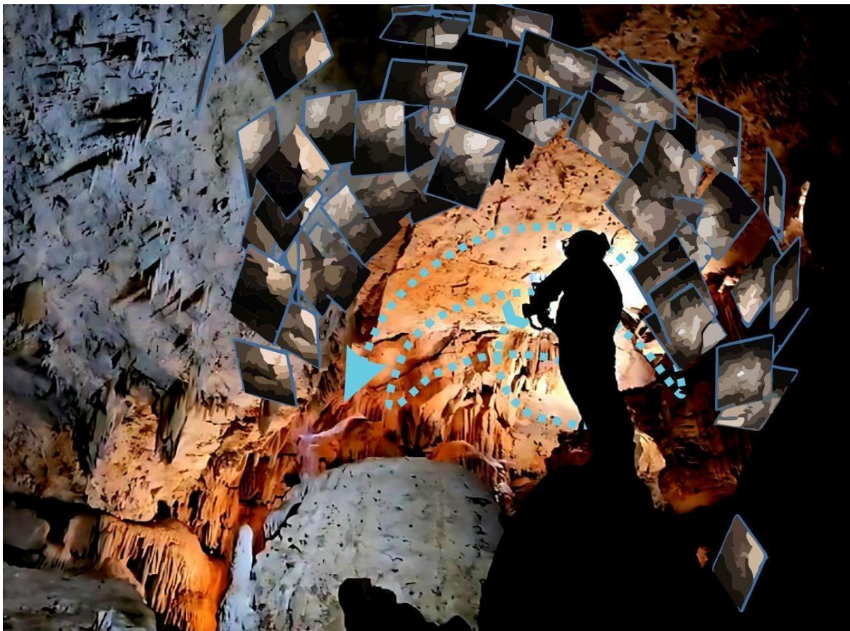
Figure 1. Representation of the photogrammetric data acquisition technique in a cave environment. The survey is based on the protocol for photogrammetric acquisition in caves, using 360° acquisition globe photographs.
