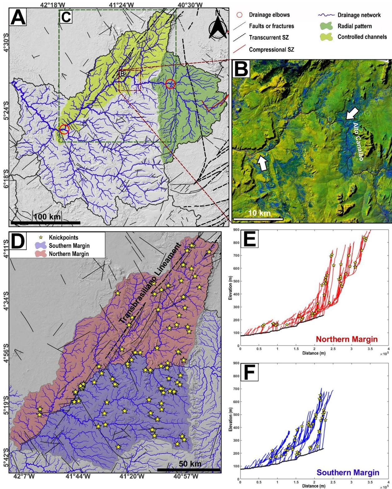
**Figure 4.** Drainage network and longitudinal profiles of Poti River. A- Drainage patterns and drainage inflexions. B – Orthogonal drainage anomalies (white arrows mark the inflexions). C – Longitudinal profiles of channels draining the middle course of the Poti River. D and F – Longitudinal profiles of the rivers in the northern (D) and southern (F) margins. Chart C indicates the location of the topographic data in Figure 5.
