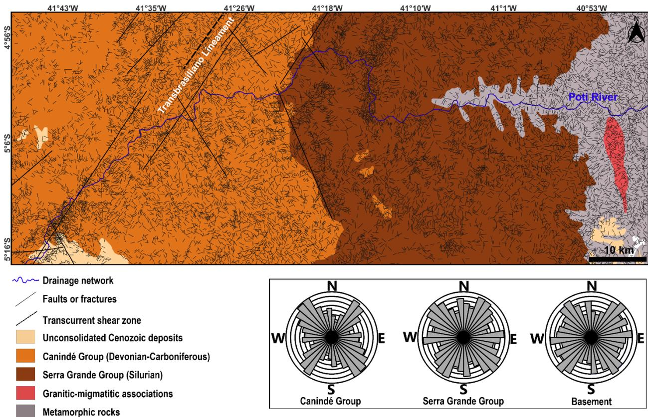
**Figure 8.** Mapping, distribution, and preferential direction (rose diagrams) of the lineaments present in the Canindé and Serra Grande Groups, and the lineaments identified in the crystalline basement.
