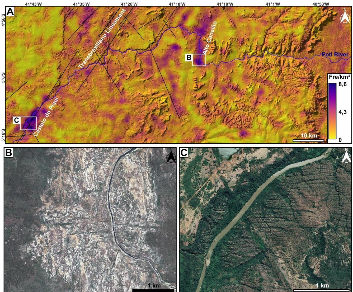
**Figure 9.** Lineament density (Frequency/km<sup>2</sup>) mapped along the Poti River Canyon (A). B and C – Rocky pavements in Alto Canalão (B) and Castelo do Piauí (C). Note the complex orthogonal fracture systems and their influences on the density values. Source: Satellite images from Geoeye-1 (Digital Globe) available in Google Earth (2023).
