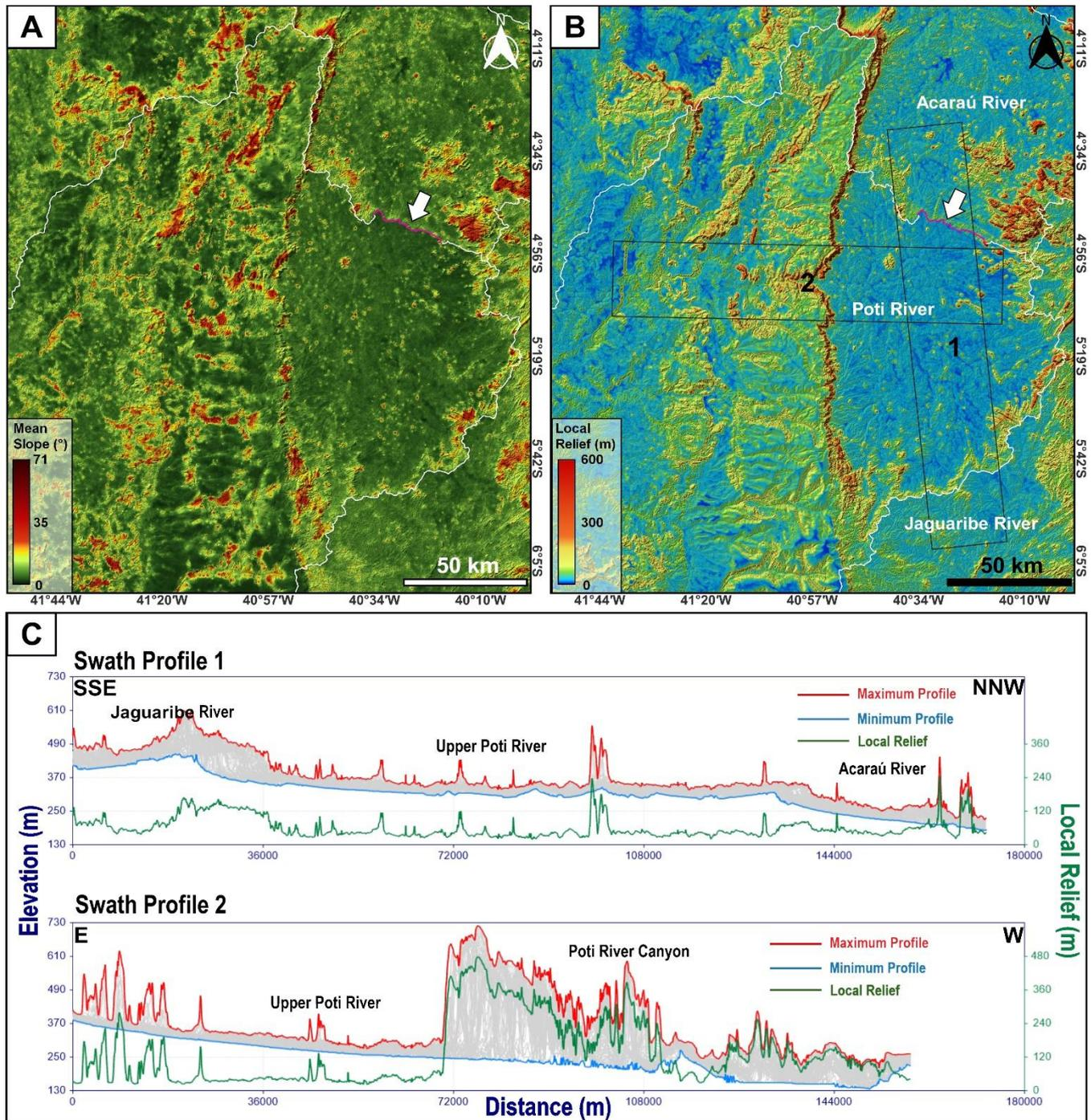
**Figure 5.** Mean Slope (a), Local Relief (B) and Swath Profiles (C) of terrains drained by Poti River. In A and B is presented a lowered segment in the divide between the Poti and Acaraú rivers (purple line indicated by white arrows).
