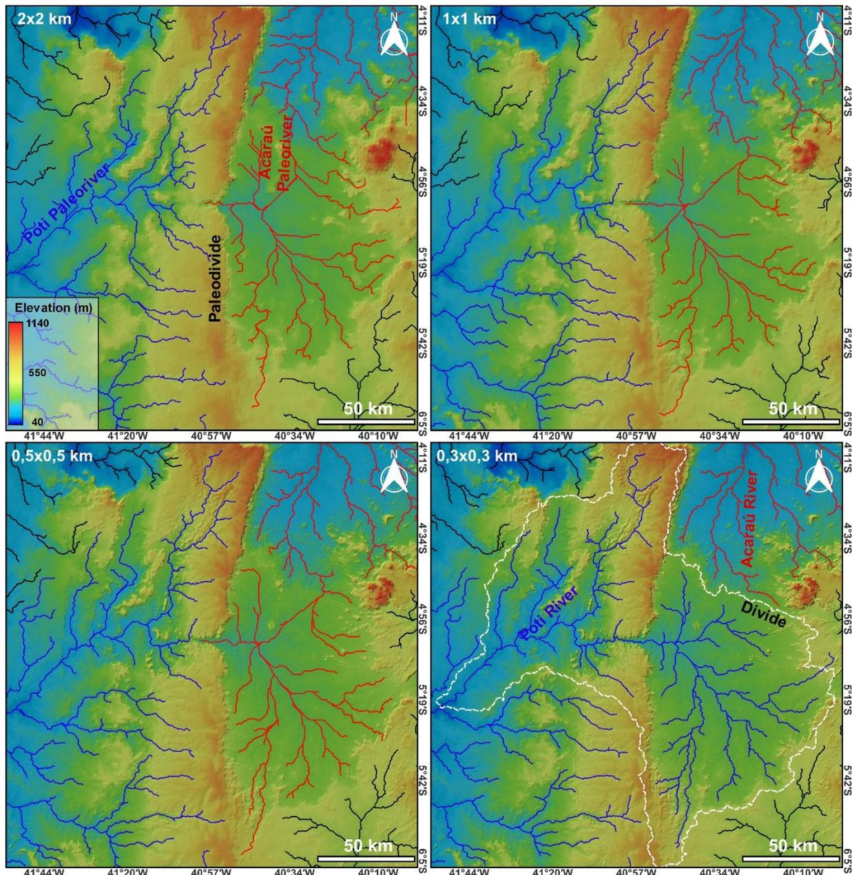
**Figure 7.** Paleotopographic models of the terrains drained by Poti River. Note that, according to the diminishing of the sample windows, the scenarios suggest a river capture involving Acaraú and Poti River.
