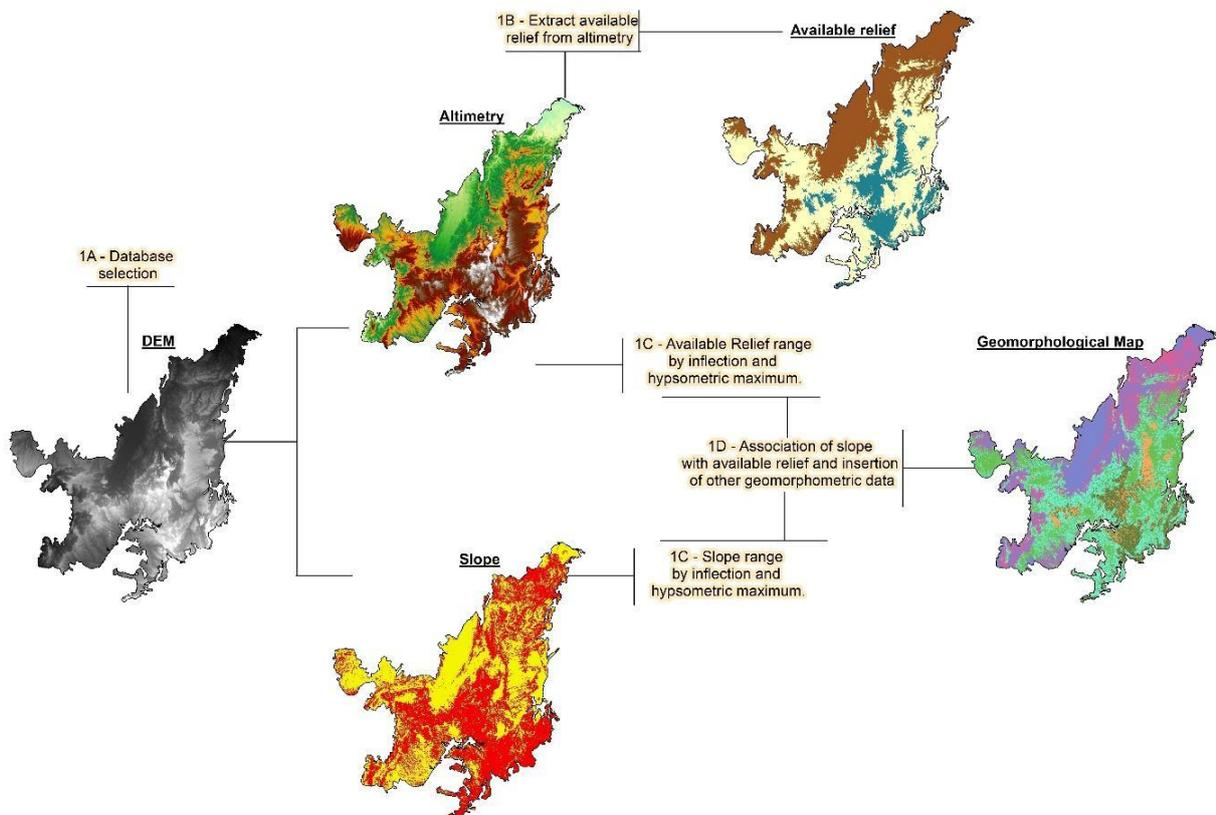
**Figure 2.** Steps of the methodological procedure. Step 2A: database selection. Step 2B: representation of the available relief from the DEM. Step 2C: delimitation of available relief and slope ranges. Step 2D: algebra of available relief ranges and slope to determine the BRUs, and insertion of other geomorphometric data, to define the geomorphological map.
