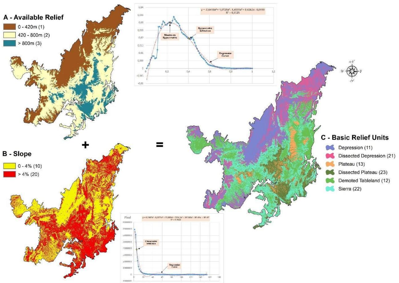
**Figure 3.** Correlations between available relief (A) and slope (B) determining the classes of Basic Relief Units (C) and graphs used to obtain the available relief's and slope's intervals. R-values higher than 0.9.
