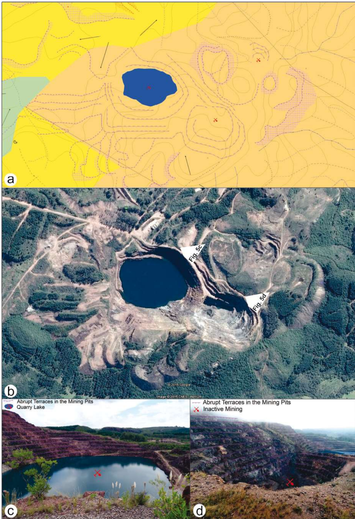
Figure 5 – Anthropogenic morphologies created from the digging/blasting step. The legend with the presented symbology in the geomorphological map excerpt and in the photography obtained in field can be seen with more details on Figure 2.
